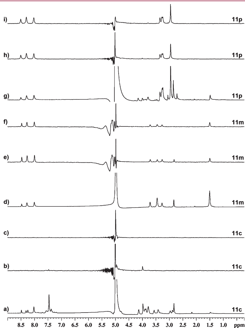
Figure 4. 1D proton spectra (a, d, g) and the corresponding STD NMR spectra recorded upon saturation at 10 ppm (b, e, h) and -1 ppm (c, f, i) of 11c /DNA, 11m /DNA, and 11p /DNA complexes, respectively. The STD NMR spectra were plotted with the same noise level.
